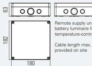
Remote supply unit for rechargeable battery luminaire for mounting in temperature-controlled indoor area
