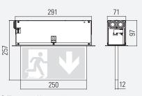
Ceiling cutout: 295 mm x 75 mm Maximum ceiling thickness: 43 mm
